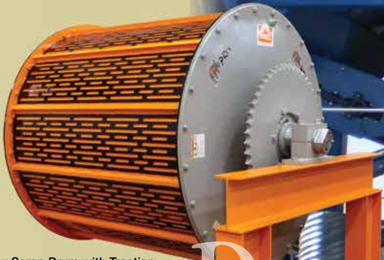
P-Rex Scrap Drum with Traction Plate Drum Wrap provides magnetic gripping power from edge to edge.
