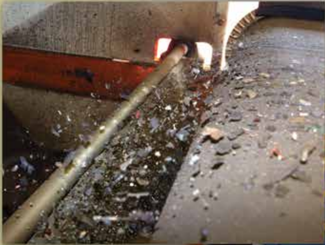
Small nonferrous metals are propelled over the splitter
