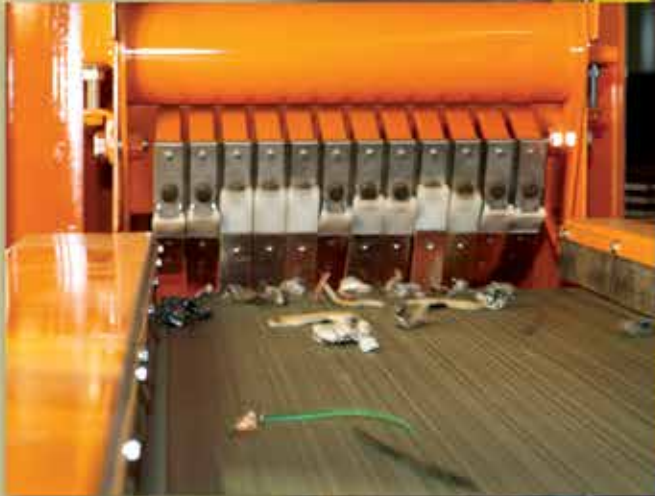
Powerful paddles deflect metals into sorting stations
